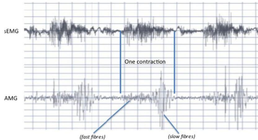
**Figure 8** A simultaneous surface electromyography (sEMG) (upper trace) and AMG (lower trace) recording from *m. Gastrocnemius* of a healthy human control subject during a period of stair descent. Note: (i) the same time frame for the start and finish of the sEMG and AMG signals, and (ii) the clear fast-fibre (low amplitude – concentric contraction) phase and the slow-fibre (high amplitude – eccentric contraction) phase, only detectable using the AMG technique.
